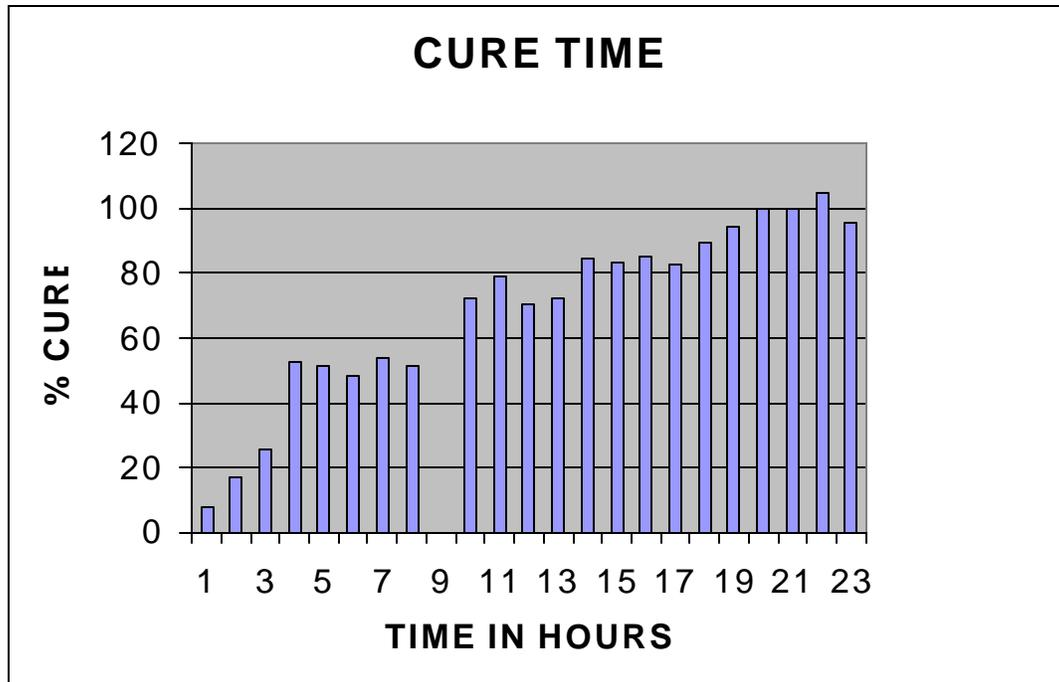
The conclusion is that the material cures to about 60% of its final strength in about 8 hours. Location L1.
