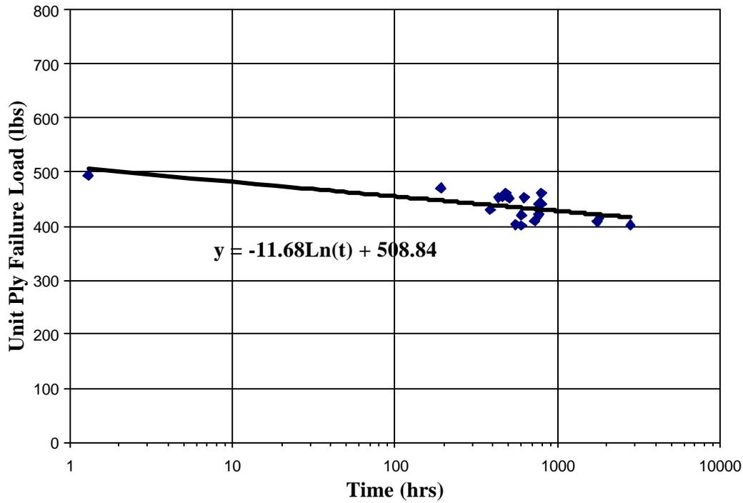
First the slope of the room and elevated temperature plots is identical and the offset between them is 9%. This indicates that the long term load handling capability at elevated temperatures had a difference of only 9%. This is an excellent result. Location L7.
