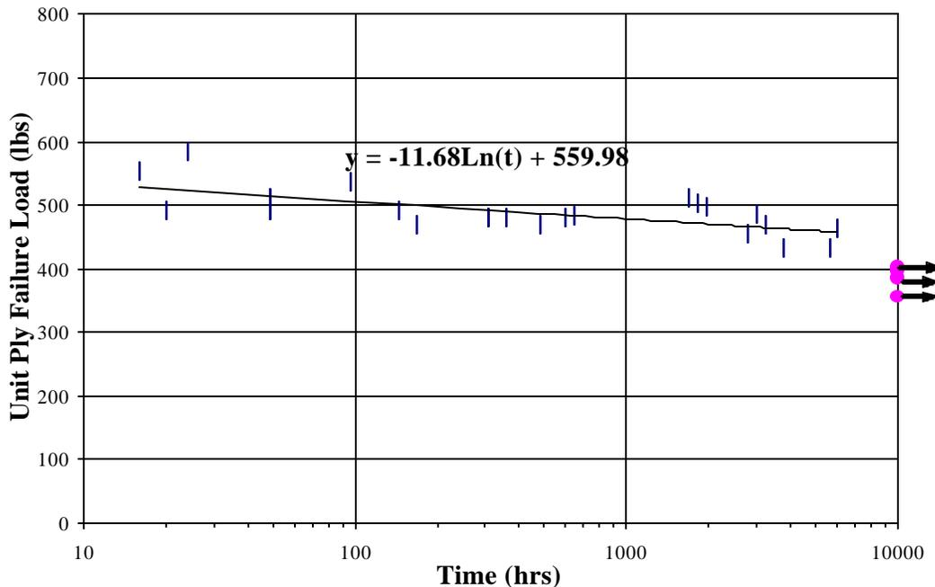
The baseline strength of this 11 oz. tape material is 801 pounds per ply. The 25-year projection of 416 pounds per inch represents a long-term load capability of 52% of its initial tensile strength.
