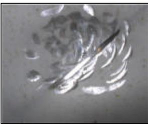
Fig. 1 – Top view of impact dent with gouge.
