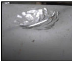
Fig. 2 – Angled view of dent with gouge.
