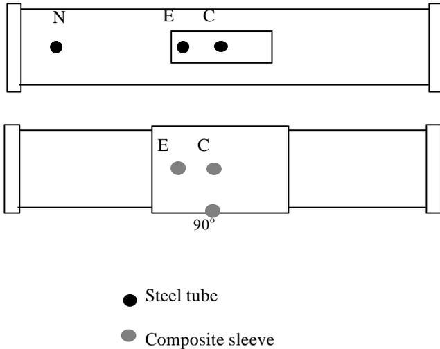
Figure 3 – Strain gage rosettes locations on the tubular specimens, both at metallic and composite surfaces.
