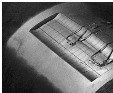
Figure 1 – External defect of a specimen without composite reinforcement, also showing the strain gage rosettes.
