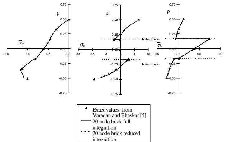
Figure 4 - Comparison between FEA and exact values, for a thick (90°/0°/90°) layered laminated tube.
