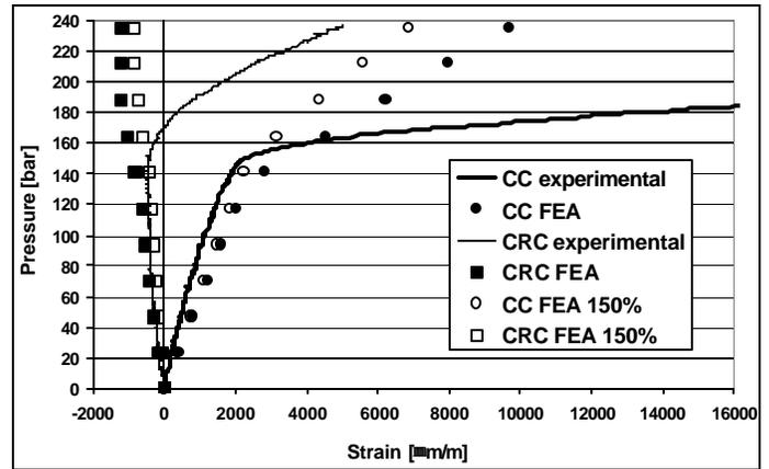
Figure 7 - Comparison between experimental and FEA results for the C repaired tube with internal defect.
