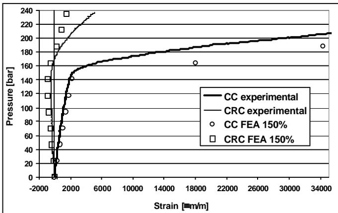
Figure 8 - Comparison between experimental and FEA results for the C repaired tube with internal defect, incorporating two hypotheses.
