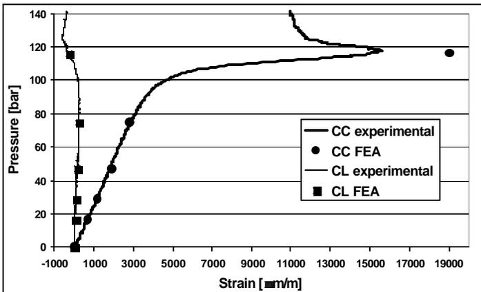
Figure 6 – Comparison between experimental and FEA results for the non-reinforced tube with external defect.
