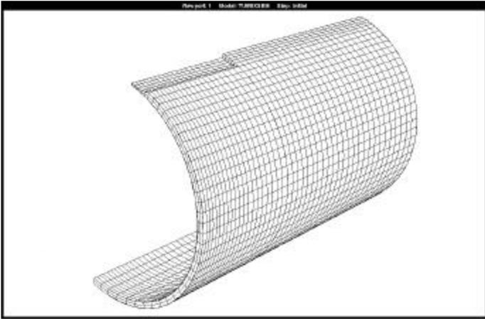
Figure 5 – Finite element mesh of the non-reinforced tube with external defect, taking advantage of the double symmetry.
