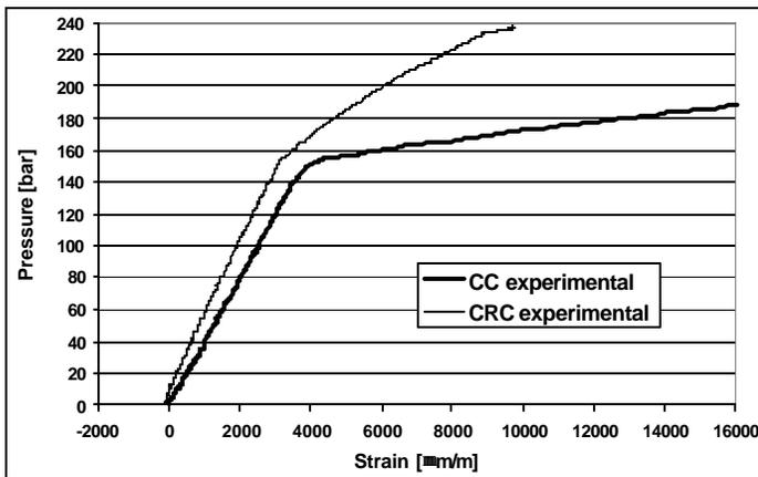
Figure 9 - Experimental results for the C repaired tube with external defect.
