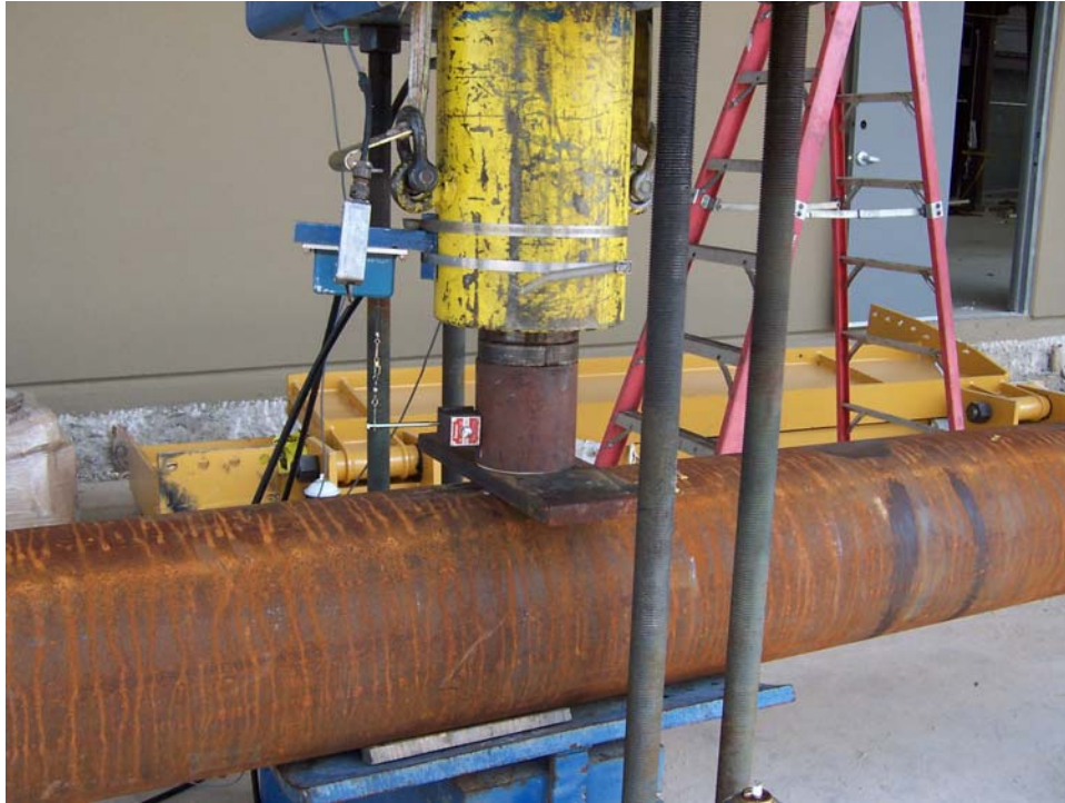
Figure 1 - Dent installation rig to install dents
