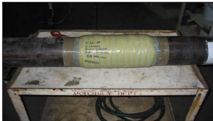
Tested to 8200 psi With No Failure per ASME PCC-2 Short Term Spool Test
